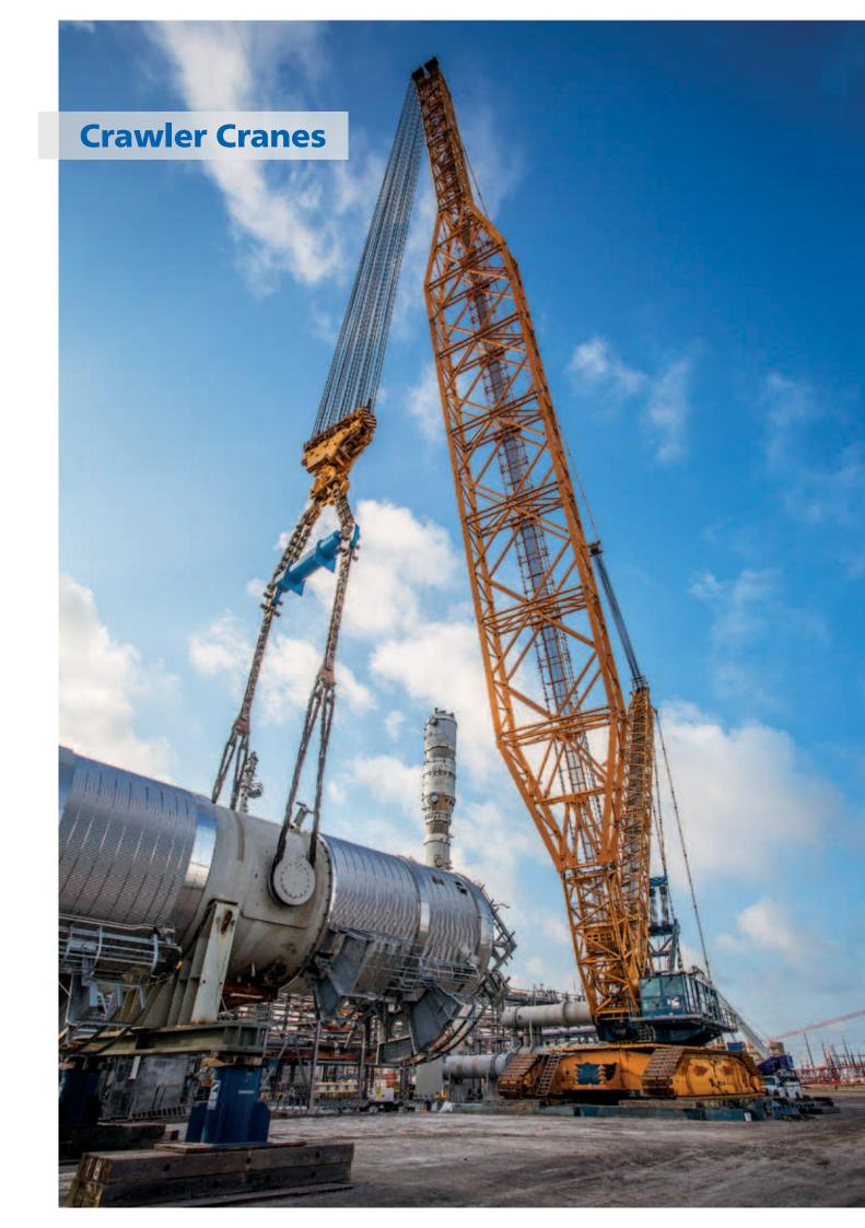
When the job demands something unusually big and powerful, consider a Demag crawler crane. They have more lifting capacities than other types of cranes – up to 3,200 t – and maintain excellent maneuverability under heavy load. Despite their size, Demag crawler cranes are easy to transport and, once at the jobsite, quickly rigged. Innovative solutions and high safety standards provide you with the right crane for every application.
