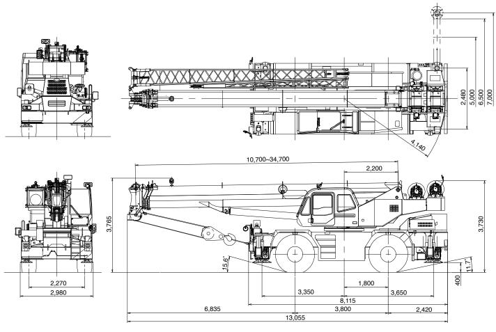
Note: Dimension is with boom angle at -0.8 degree.
