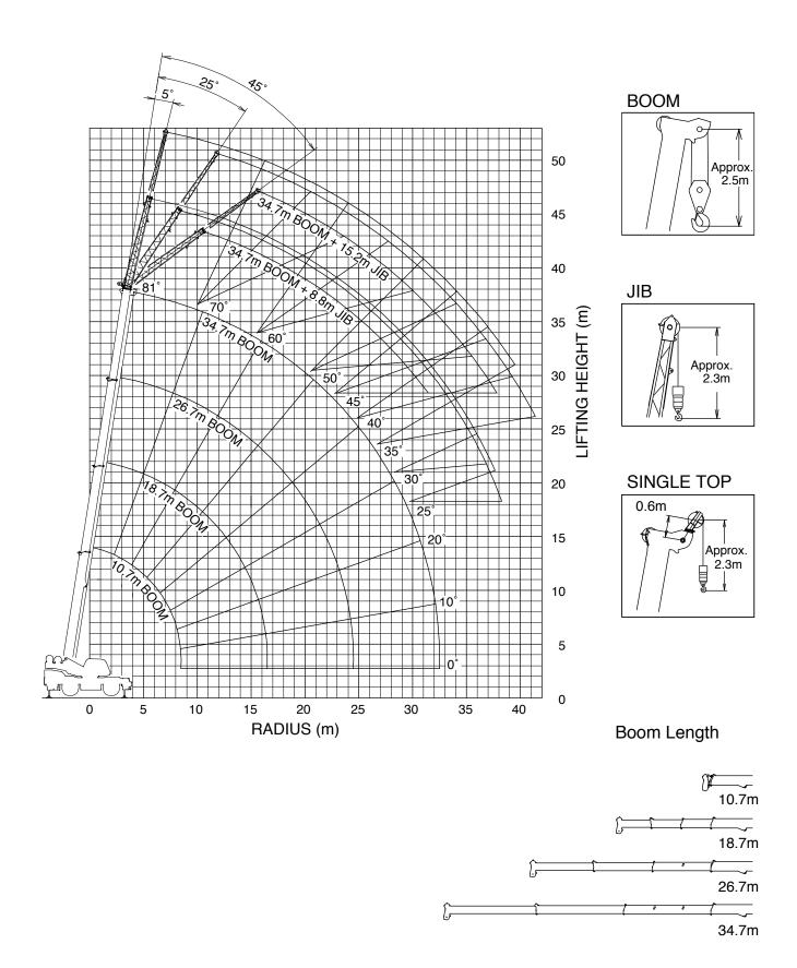
**NOTE:** The above lifting height and boom angle are based on a straight (unladen) boom, and allowance should be made for boom deflection obtained under laden conditions. The above working range is shown on condition with outriggers fully (7.0m) extended.
