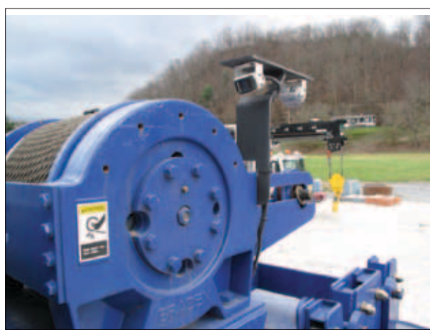
Cameras display the winch as well as the blind area directly behind the crane. Full color video display in operator cab is standard equipment.
