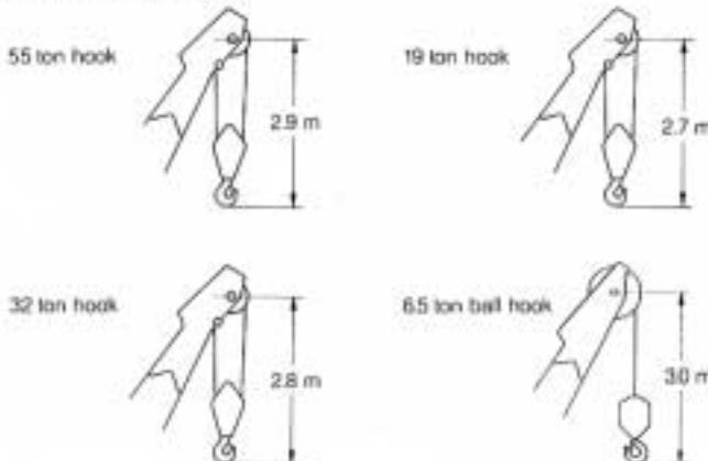
NOTE: These lengths are recommended for boom and jib angles of 75° or less.
