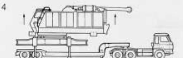
The upper frame is turned 90°, the translifter jack cylinders are further extended, and a trailer is positioned beneath the carbody.
