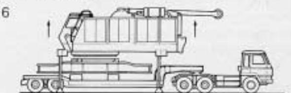
The upper is supported by upper translifter and carbody is separated by "Quick undocking device".
