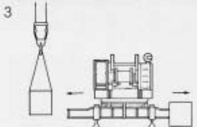
The horizontal cylinders push the crawler frames out, and each crawler frame is lifted with the auxiliary crane 45 tons or larger.
