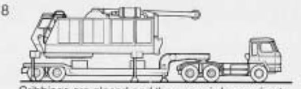
Cribbings are placed and the upper is lowered onto the trailer.
