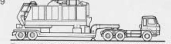
The translifter jack cylinders are fully retracted inside the upper frame.
