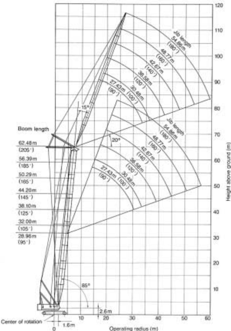
**Luffing jib rated loads in metric tons—360° work area (boom angle: 85°)**
