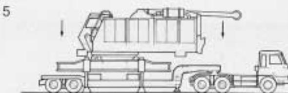
Cribbings are placed, and the machine is lowered onto the trailer.
