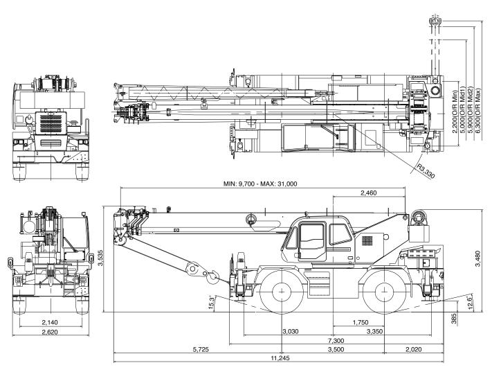
Note: Dimension is with boom angle at 0 degree.
