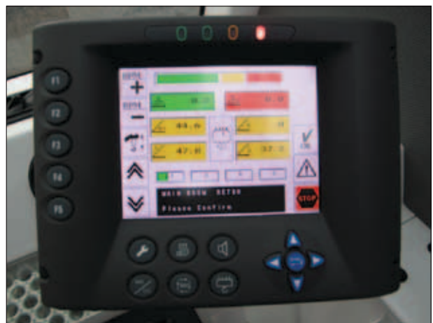
State-of-the-art, user friendly rated capacity limiter provides continuous feedback of crane lift and position data.
