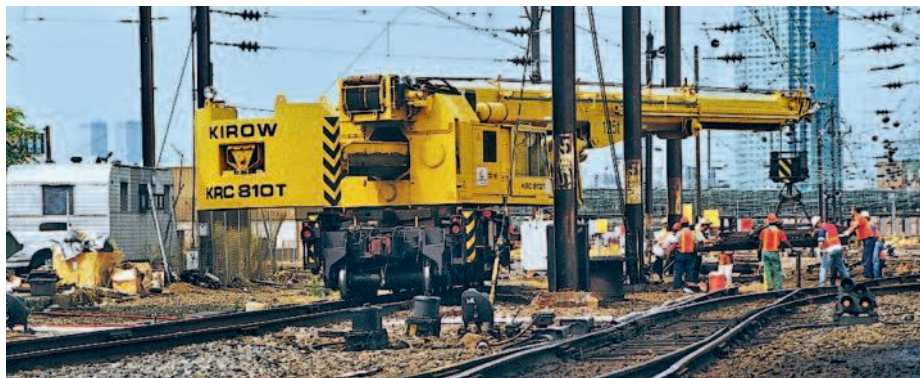
↑ Telescopic boom for high flexibility of application
