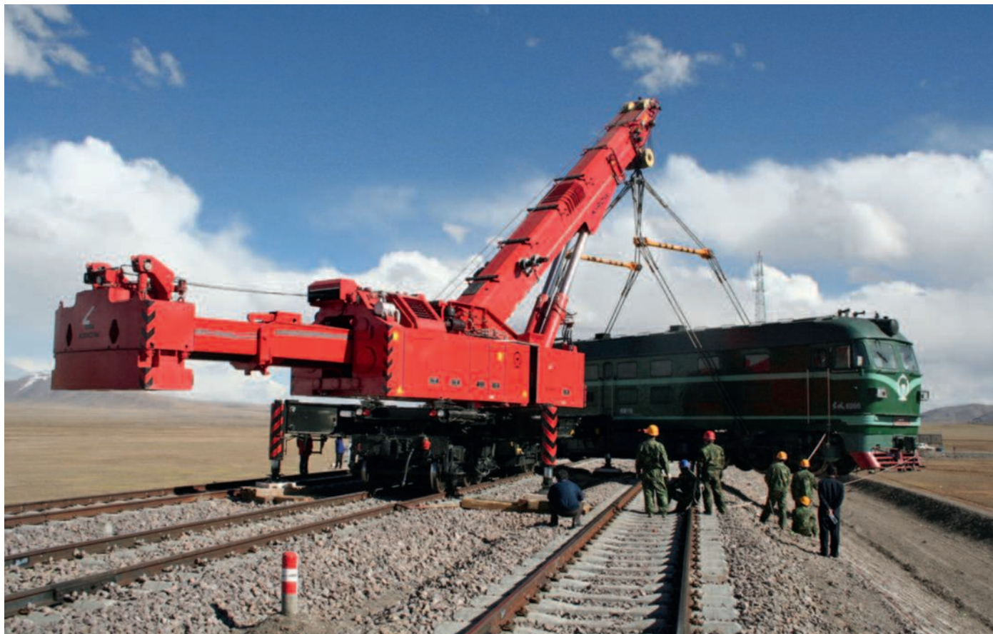
Multi Tasker 1600 during recovery of a locomotive in Tibet
