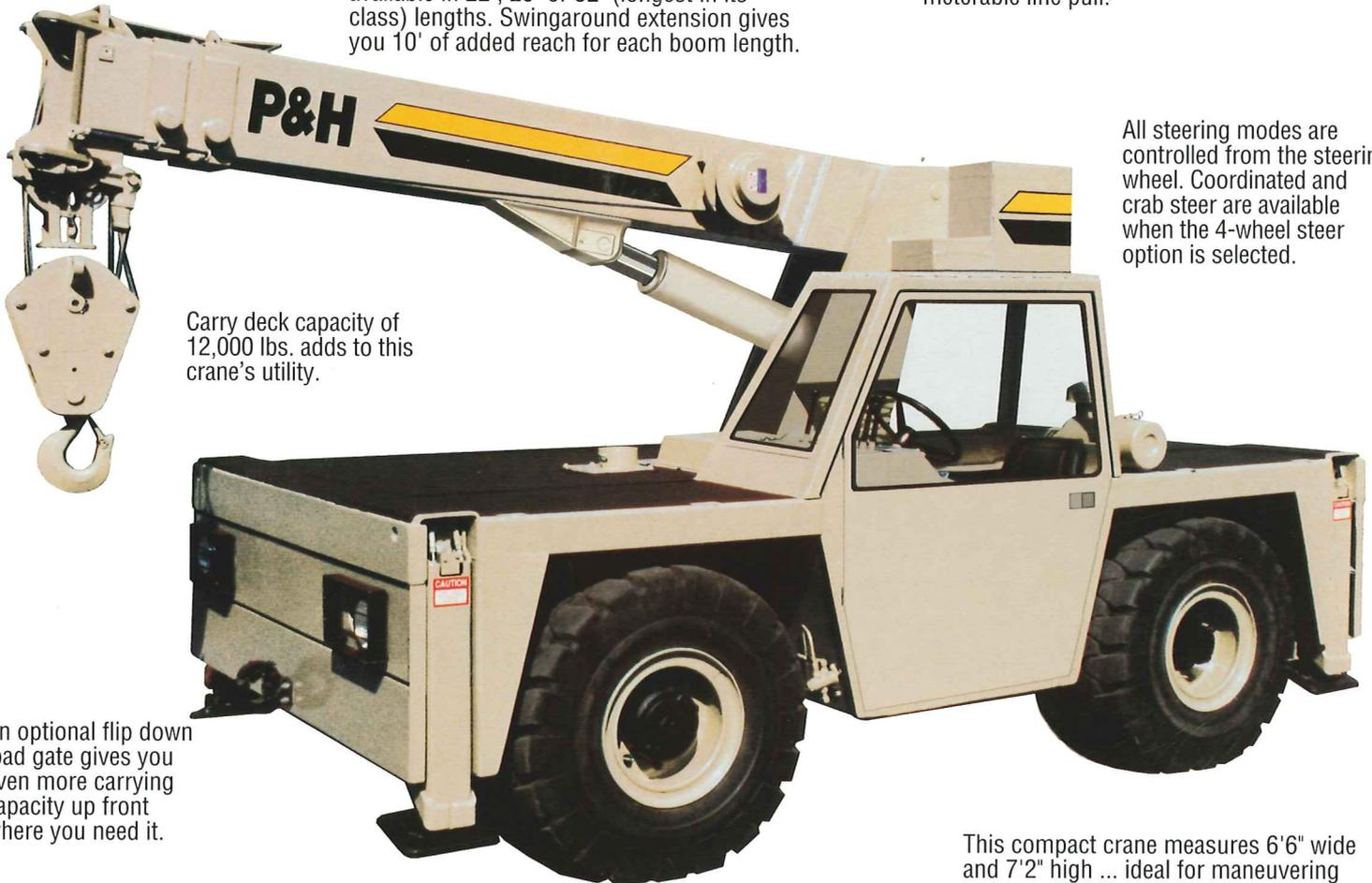
Carry deck capacity of 12,000 lbs. adds to this crane's utility.
