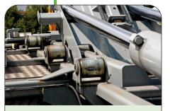
The Hyva Lift hookloaders are delivered with container supporting rolls for quiet and easy loading of the containers. Two rear rollers, which support the container's lower frame, have bronze bearings.
