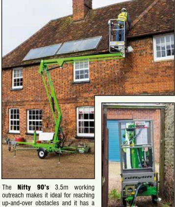
telescopic axle to allow it to pass through a 0.9m (2ft 11in) opening.
